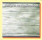
The surface of the cylinder is worn, scratches and risks are 0.1 mm in depth.
