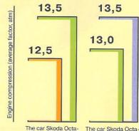
The car Skoda Octavia, year of production: 1999, mileage in the beginning of the test: 40,260 km. After the mileage of 57,500 km with regular semi-synthetic oil SAE 10W-40 API SJ/CF, the compression reduced.
